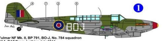
Fulmar NF Mk. II, BP 791, BO-J, No. 784 squadron FAA, RAF Drem, Lothian, late 1944 Aircraft in non-standard camouflage of Medium Sea Grey overall with Dark Green fields. Note the White line behind fuselage rounded on left side.
