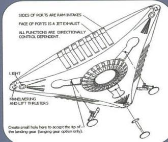
STEP 2: Glue landing gear to Lower Saucer Half, if desired.
