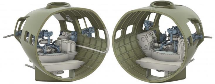
B-17G Early Production Bombardier position & Chin turret
